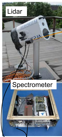
Fig. 1: Instrumental setup of LIRAS
