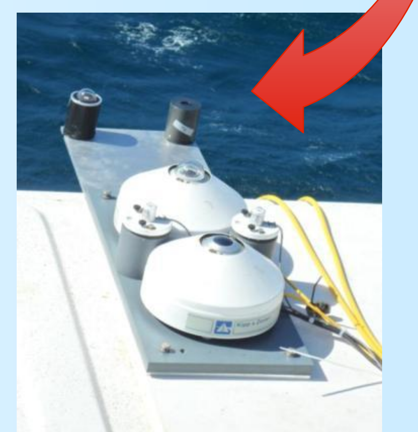
Fig. 3: Optical inlets from CORAS and Pyrano- and Pyrgeometer
