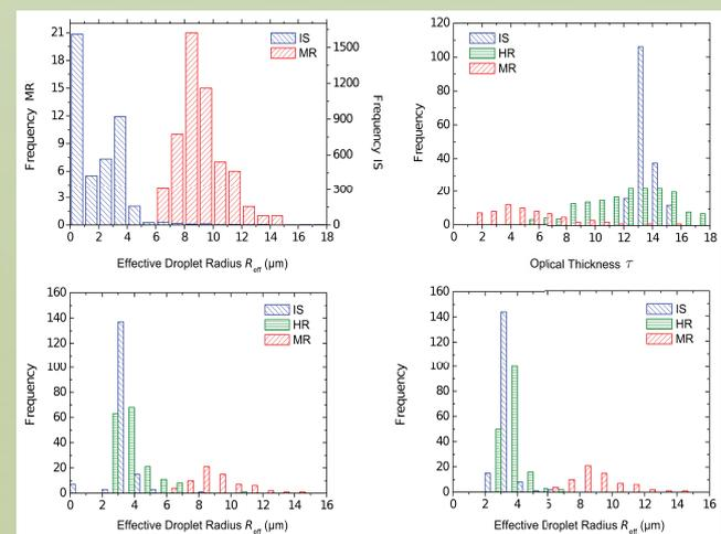
Fig. 5: Histogram of in situ measurements (IS) and MODIS retrieval (MR) of  $R_{eff}$  for the full flight track (top-left panel) and including the retrieval from the radiation measurements on the helicopter (HR) for CC1 (bottom-left panel) and CC2 (bottom-right panel). (Top-right panel): Histogram of IS, HR and MR of  $\tau$ .
