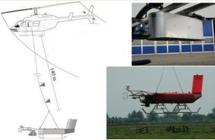
Fig. 1: The radiation instrumentation is installed underneath the helicopter and ACTOS is carried by means of a 140 m long rope. One close-up shows the housing of the optical inlets for upwelling irradiance  $F_{\lambda}^{\uparrow}$  (transparent semi-spheres) and radiance  $I_{\lambda}^{\uparrow}$  (flat opening). A photo of ACTOS is shown on the bottom-right side.
