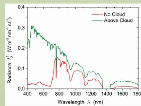
Fig. 2: Examples of spectra of upwelling radiances  $I_{\lambda}^{\uparrow}$  for cloud-free conditions and above a cloud.
