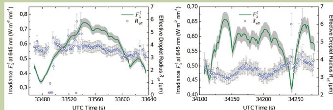
Fig. 3: Time series of in situ measured effective droplet radius  $R_{eff}$  from the PVM and upwelling irradiance  $F_{\lambda}^{\uparrow}$  for CC1 (left panel) and CC2 (right panel). The grey areas and error bars indicate the measurement uncertainties for the radiation measurements and the in situ measured  $R_{eff}$  from the PVM, respectively.
