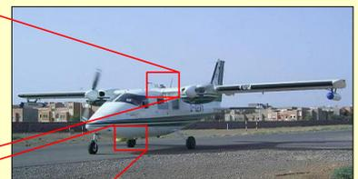
Fig. 1: The Partenavia P68B research aircraft at Ouarzazate airport (top), and a close-up of the optical inlets (left) for irradiance (transparent semi-spheres) and actinic flux density (whitish heads). The grey cupola holding the inlets is automatically tilted for fast and accurate horizontal stabilisation during flight.
