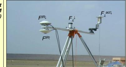
Fig. 3: The surface spectrometer inlets. From left to right: Thermal broadband sensors, irradiance inlet, actinic flux density inlet.
