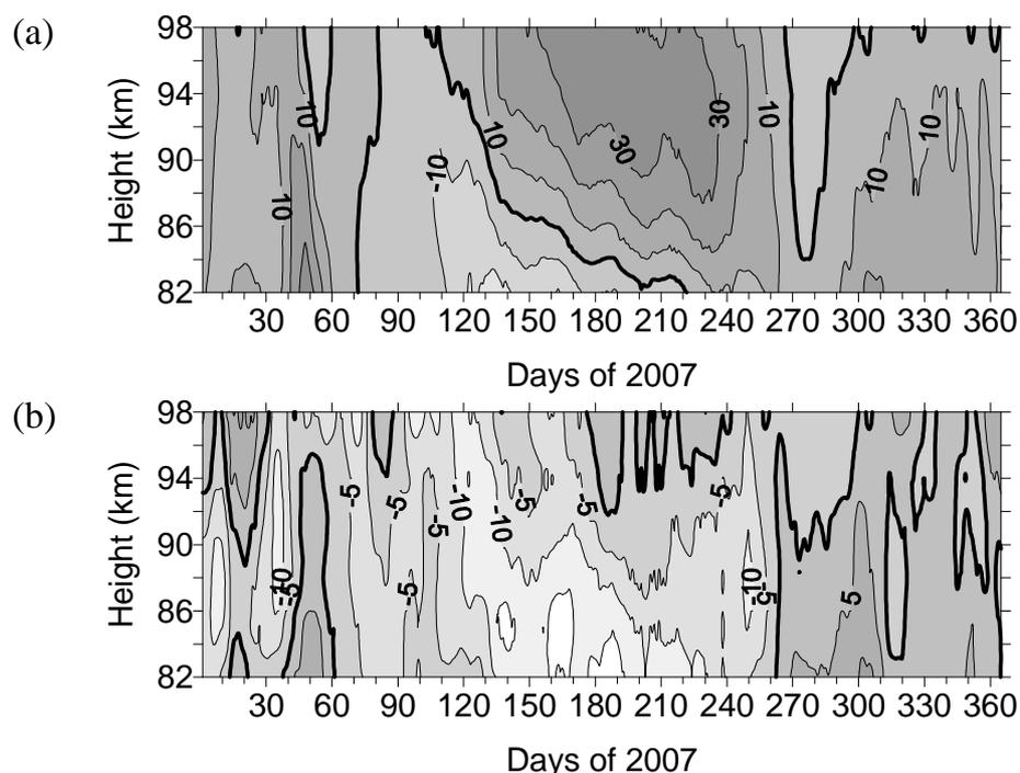
Figure 1: *Height-time cross-sections of the (a) zonal and (b) meridional prevailing winds as measured by the Collm meteor radar. Data base on multiple regression analyses including 15 days of hourly winds each.*
