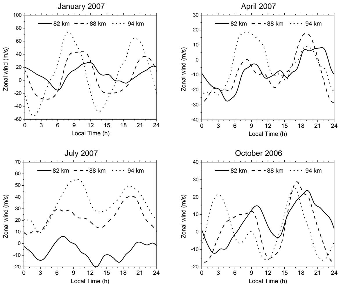
Figure 3: Monthly mean zonal winds at 3 different height gates, measured with meteor radar at Collm, for 4 seasons. Note the different scaling of the ordinate in the respective panels.
