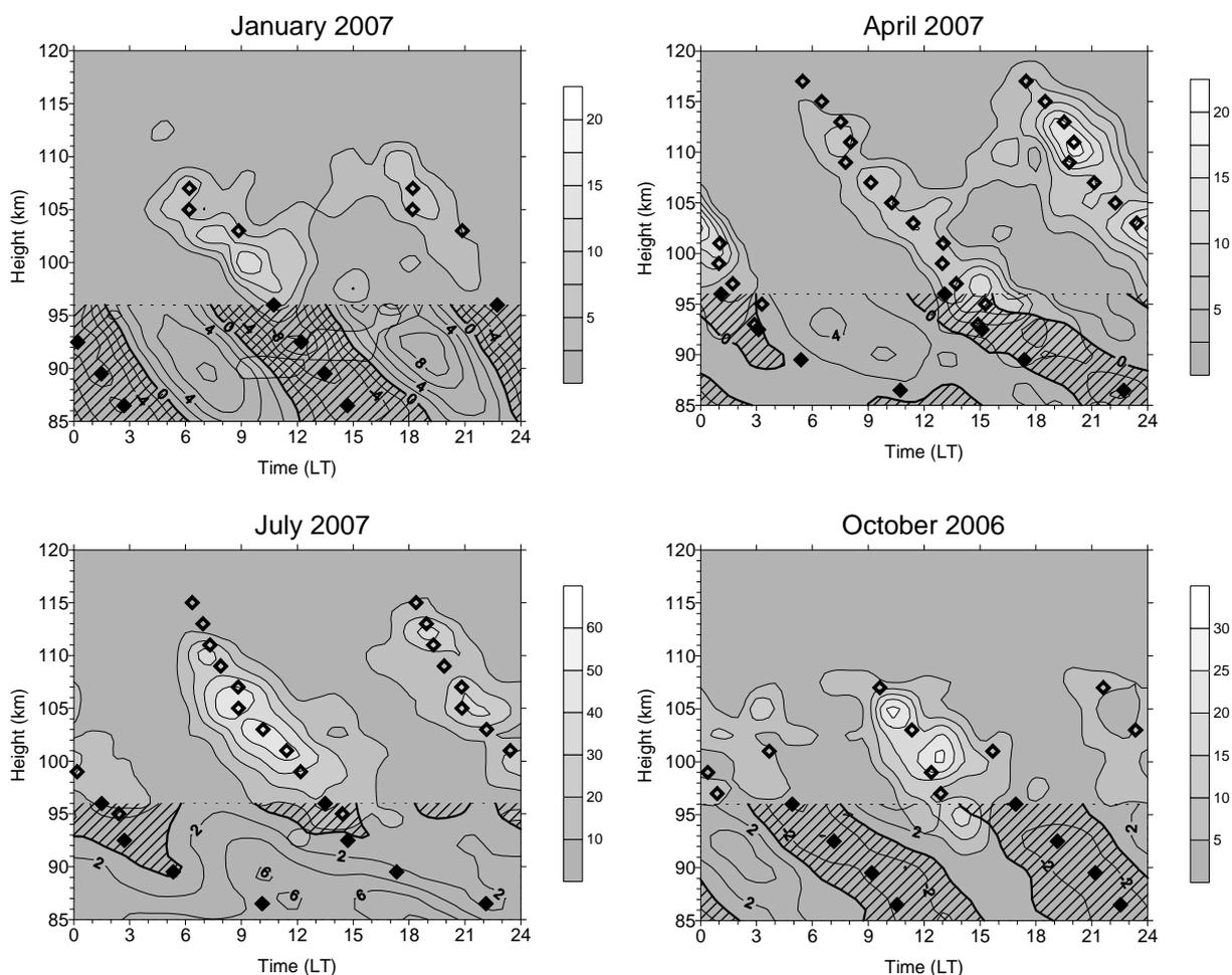
Figure 4: FORMOSAT-3/COSMIC relative Es layer occurrence (in 1/1000), for a latitude range from 50°-55°N (greyscaling). In the lower part monthly mean wind shears, given in  $\text{ms}^{-1}\text{km}^{-1}$ , measured with the Collm meteor radar are shown as isolines. Negative shear values are hatched. Added are SDT phases of Es layer occurrence (open symbols) and wind shear (solid symbols, phase is defined as time of minimum shear).
