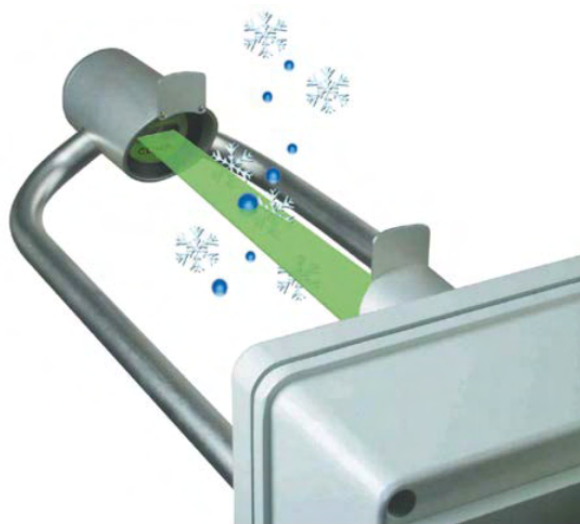
Figure 1: Measurement principle of the optical disdrometer by Thies - Hydrometeors like snow or rain cause an attenuation of the laser beam while falling through the beam. Based on the extent and duration of the attenuation the hydrometeor size and velocity are estimated. [Adolf Thies GmbH & Co KG, 2015]
