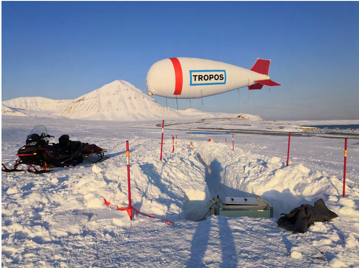
Figure 1: The balloon site as observed on 28 March 2022. The winch in the foreground controls the vertical release of the balloon. The tether is uncoiled horizontally towards a deflection pulley located underneath the balloon in the background. The extensive snow cover allowed for the use of snowmobiles in logistics operations.
