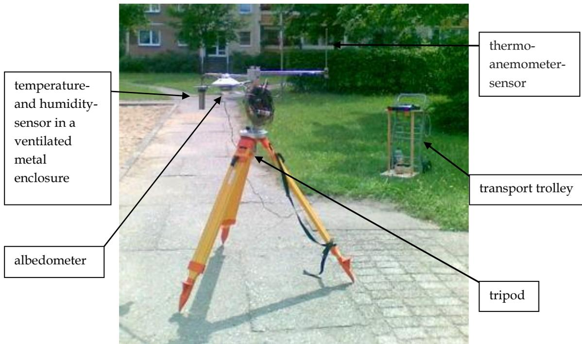
**Figure 1:** *Measurement setup, positioned at a measuring point in Leipzig-Paunsdorf.*
